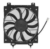
To prevent damage if a cooling fan gets blocked, the circuit powering the fan needs a time-delay type fuse with the correct amperage rating. This installation uses 1x suction fan - part number FAN0089 (F07P-12E8004-02S). The nominal running current is 8.1 amps.
